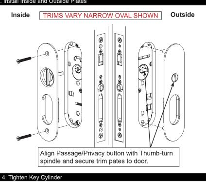
Tighten locking screw to engage notches on cylinder
