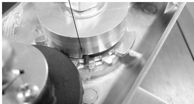
Spring orientation for right hand reverse operation
