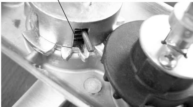
Spring orientation for right hand reverse operation
