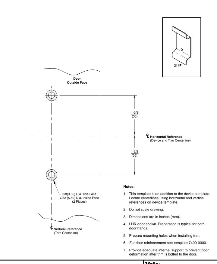
214F Trim Application for Metal Doors with 2100(F) Series Rim and Vertical Rod Exit Devices
